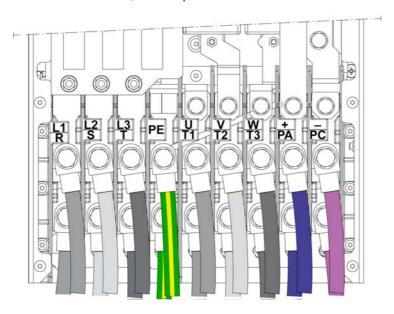
PA/+ and PC/- terminals are used to connect the braking unit. Refer to the braking unit instruction sheet <a href="https://www.schneider-electric.com">www.schneider-electric.com</a>.
