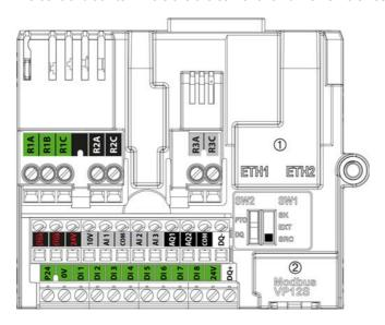
① Ethernet Modbus TCP, ② Serial Modbus
