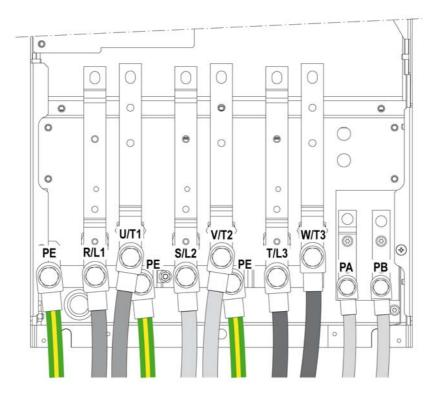
PA/+ and PB terminals are used to connect a braking resistor. Refer to the braking resistor instruction sheet <u>NHA87388</u> available on <u>www.schneider-electric.com</u>.
