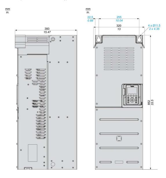
IP21 / UL Type1 Drives - Front, Rear and Side View
