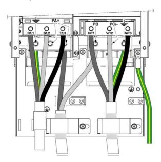
PA/+ and PB terminals are used to connect a braking resistor. Refer to the braking resistor instruction sheet <u>NHA87388</u> available on <u>www.schneider-electric.com</u>.
