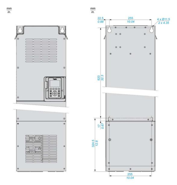
**NOTE:** Lower Conduit Box part sold separately. This part enables wall mounting of the product. It provides IP21 protection degree on the bottom side and UL type 1 protection degree.
