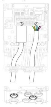
**NOTE:** Cabling plate shown is for frame size 2. Other cabling plates look slightly differs from this one. **NOTE:** For Floor standing products route the option cables into the integrated control cable conduit.
