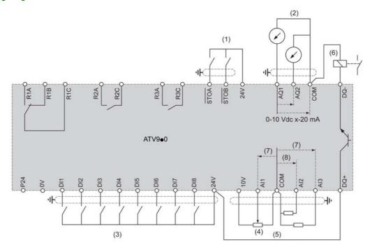
(1) STO Safe Torque Off, (2) Analog Output, (3) Digital Input - Shielding instructions are given in the Electromagnetic Compatibility section *(see page 172)* (4) reference potentiometer (ex. SZ1RV1002), (5) Analog Input, (6) Digital output, (7) 0-10 Vdc, x-20 mA, (8) 0-10 Vdc, -10 Vdc...+10 Vdc.
