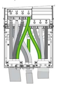
PA/+ and PB terminals are used to connect a braking resistor. Refer to the braking resistor instruction sheet <u>NHA87388</u> available on <u>www.schneider-electric.com</u>.
