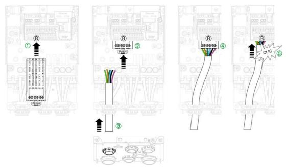
**NOTE:** Cabling plate shown is for frame size 2. Other cabling plates look slightly differs from this one. **NOTE:** For Floor standing products route the option cables into the integrated control cable conduit.
