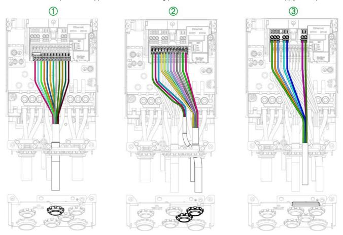
**NOTE:** Cabling plate shown is for frame size 2. Other cabling plates look slightly differs from this one. **NOTE:** For Floor standing products route the control wires into the integrated control cable conduit.
