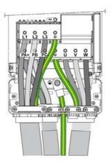
PA/+ and PB terminals are used to connect a braking resistor. Refer to the braking resistor instruction sheet <u>NHA87388</u> available on <u>www.schneider-electric.com</u>.
