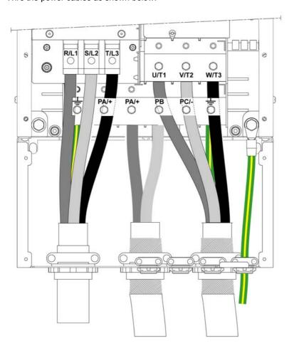
PA/+ and PB terminals are used to connect a braking resistor. Refer to the braking resistor instruction sheet <u>NHA87388</u> available on <u>www.schneider-electric.com</u>.
