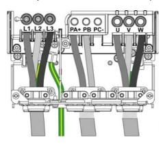
PA/+ and PB terminals are used to connect a braking resistor. Refer to the braking resistor instruction sheet <u>NHA87388</u> available on <u>www.schneider-electric.com</u>.
