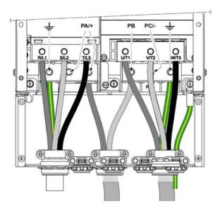
PA/+ and PB terminals are used to connect a braking resistor. Refer to the braking resistor instruction sheet <u>NHA87388</u> available on <u>www.schneider-electric.com</u>.
