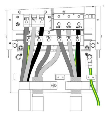
PA/+ and PB terminals are used to connect a braking resistor. Refer to the braking resistor instruction sheet <u>NHA87388</u> available on <u>www.schneider-electric.com</u>.
